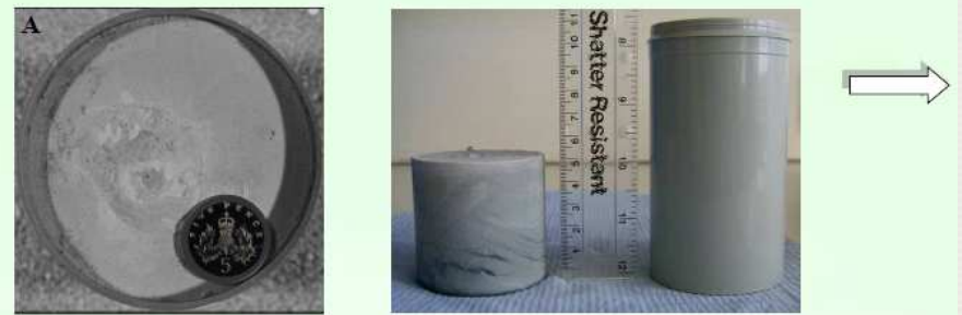
Blast Furnace Slag (BFS)/OPC (to mass ratio 7:3) with encapsulated Al
